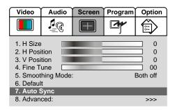
The [Auto Sync] item can not be accessed unless the unit is in VGA mode. The "Auto Adjust" function only works in VGA mode.
